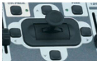
Joystick patcheable para PAN/TILT.
