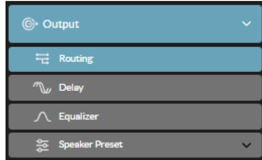
The Output Tab enables amplifier outputs to be named, linked to zones, and provides access to Delay, Equalizer and Speaker Preset menus.
