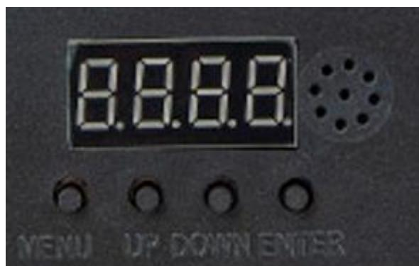
Press the MENU button once to enter MENU, use the UP and DOWN buttons to move to the desired function (according to the following chart), and press OK to confirm your selection.
