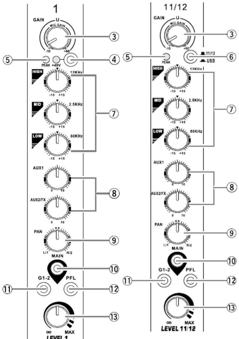
AUX(2/FX) knob controls the adjust of signal level sent to the AUX bus and FX BUS (built-in in effects). The same signal level is sending to the AUX and FX buses connected to these knobs.
