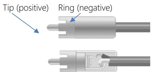
RCA interface and 1/4-inch TS interface are unbalanced interfaces. A multi-stand shielding conductor may be installed on both ends of unbalanced connection.
