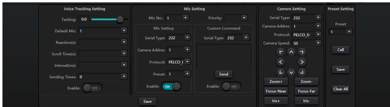
Voice tracking; set **tracking** threshold: detect microphone input signal greater than or equal to tracking threshold, the system automatically enables tracking parameters.
