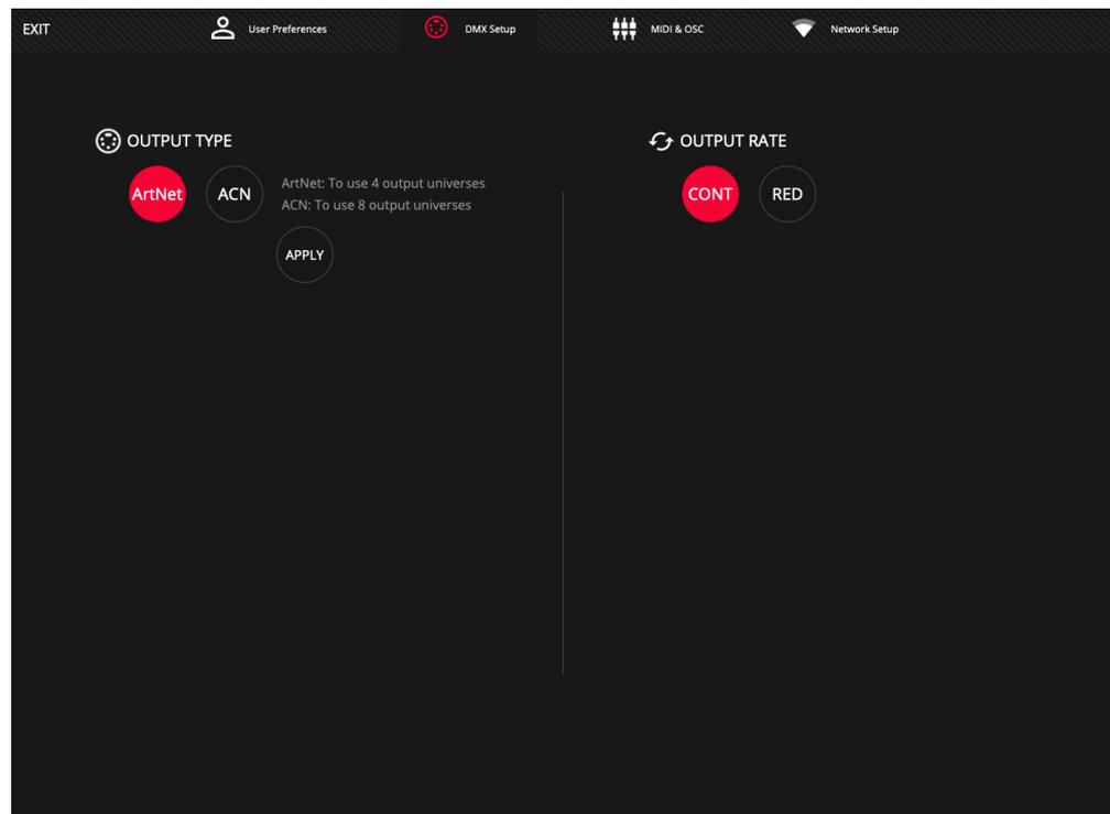
**Output Type:** Allows you to adjust the DMX output network protocol. Art-Net allows the use of up to 4 DMX output universes while ACN (sACN) allows the use of up to 8 DMX output universes.
