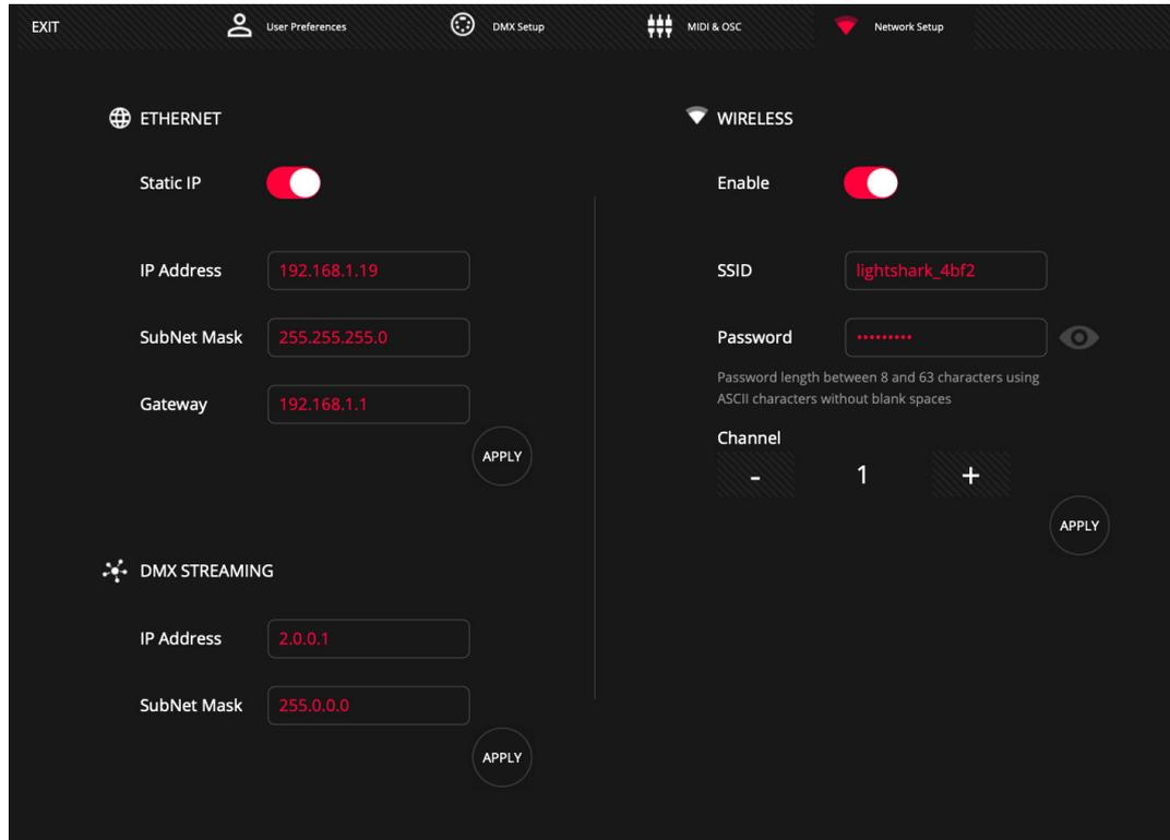
**Wireless:** Enables configuration of the integrated access point in lightShark devices. By default the network name is lightshark\_XXXX, where XXXX refers to the last 4 digits of the MAC Address of the lightShark wireless interface.
