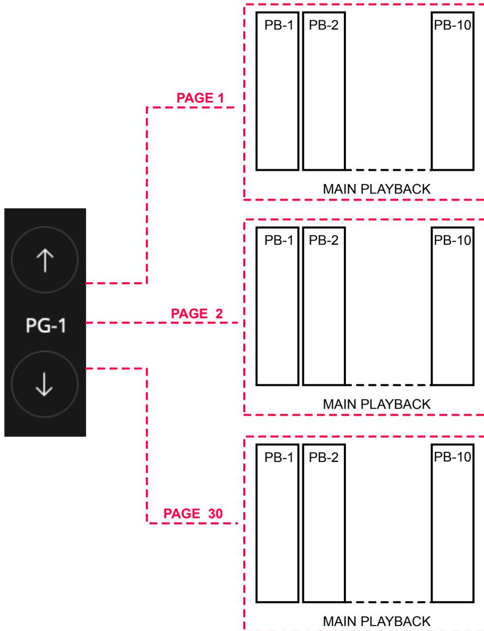
With the UP and DOWN buttons you can navigate between the pages. Between the two buttons is the label indicating the current page.
