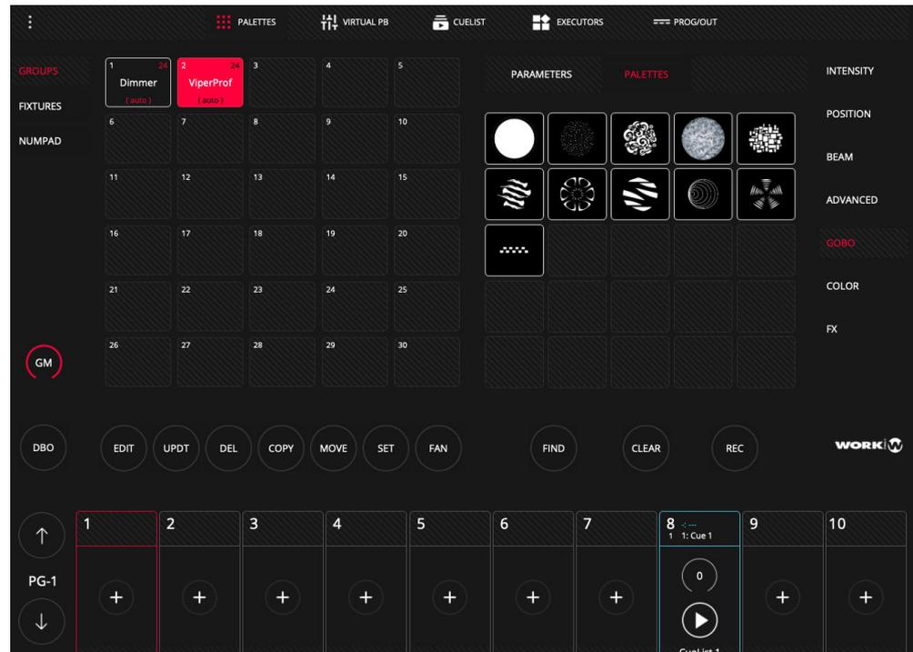
LightShark displays up to 25 pallets simultaneously, it is possible to perform vertical scrolling as in the parameter window to access more pallets.
