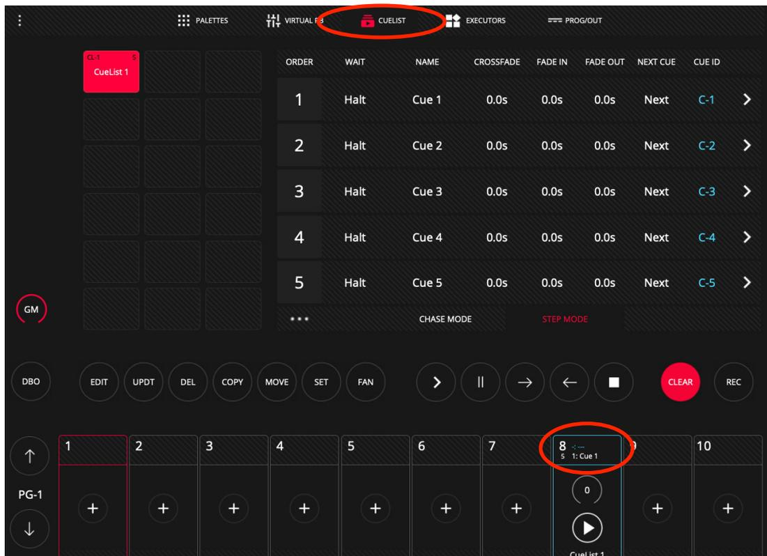
Each Cue has a Crossfade time where you can define a Fade In time and a Fade Out time.
