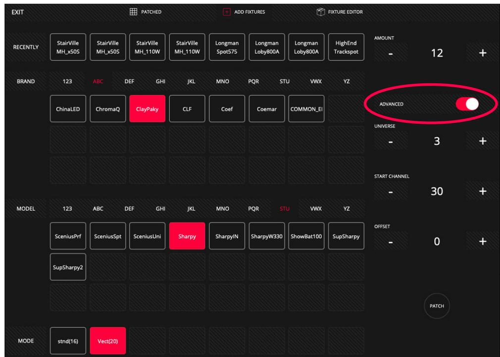
In the "Universe" field lightShark shows the number of the currently selected universe. If you want to add the fixtures in a different universe, use the + and - buttons to select the appropriate universe. If you hold down the numeric field, the on-screen keyboard will be displayed where you can directly enter the universe number.
