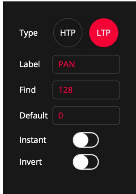
Enabling the "INSTANT" option will ignore the fade and transition times. Enabling the "INVERT" option will cause lightShark to invert the output values for that channel.
