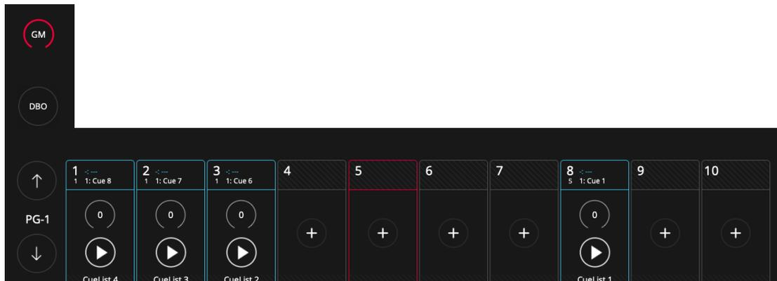
By default the GrandMaster is minimized. Click on the button to enlarge it and show the fader. Pressing it again will minimize it.
