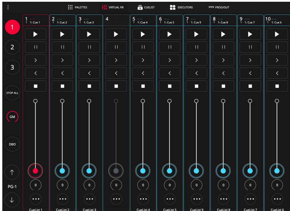
LightShark's interface is multi-touch, so you can operate multiple Playbacks simultaneously from one tablet or device. From the side buttons 1, 2, and 3 the user can directly access the desired Wing without scrolling.
