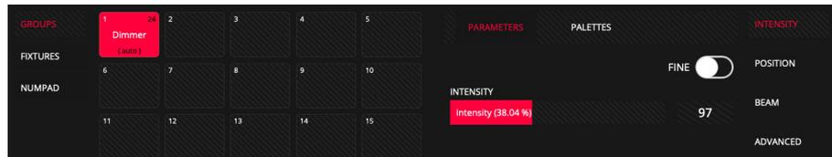
**8** You can adjust the level via the graphical interface or with encoder A if you are using an LS-1.
