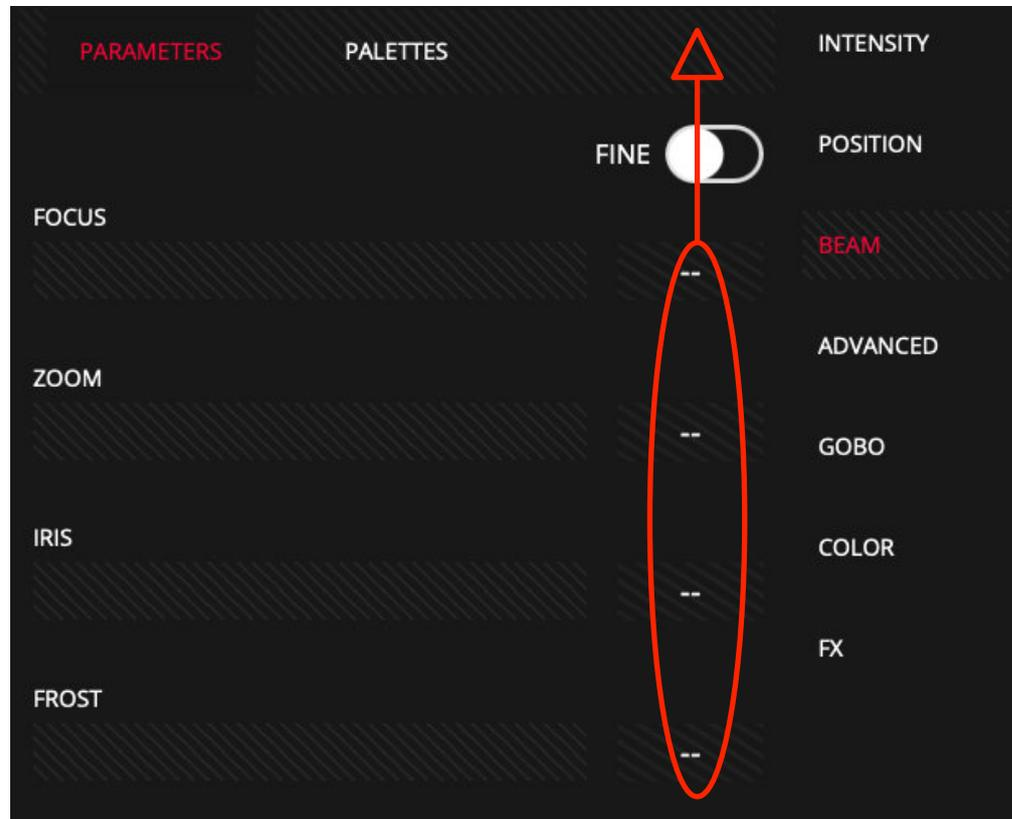
Users with an LS-1 can interact with the interface using the encoders and buttons, so that each LS-1 encoder controls each of the currently visible interface parameters (the upper parameter is controlled by the first encoder starting from the left, and so on).
