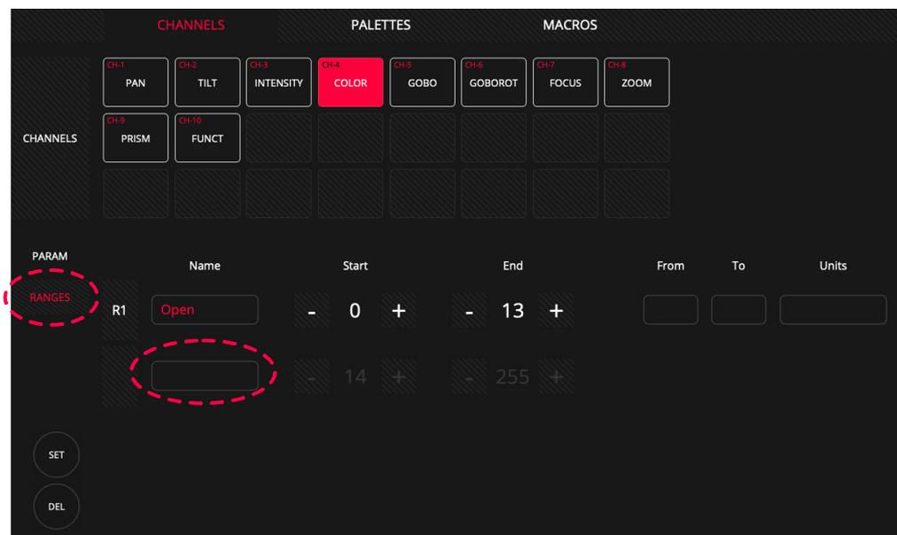
Hold down the "Name" field for two seconds to add a new segment, through the spinners set the minimum and maximum value of that range.
