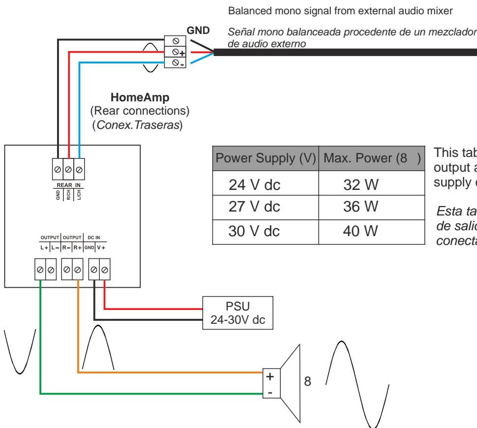
This table shows the max. power output at 8 according to the power supply connected to the **HomeAmp**.
