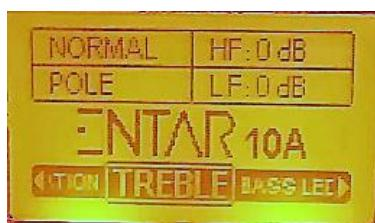
When you turn on the active loudspeaker, the display shows a basic information about some of the configurable parameters.
