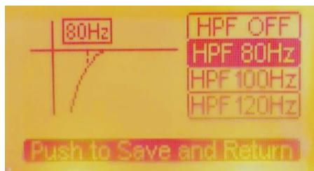
With this function, is possible to add a HPF with different cut frequency. Press and select, OFF to disable the filter, or select the cut frequency: 80 Hz / 100 Hz or 120 Hz. The response will be showed in the display. Once selected the filter, press the knob again to confirm.
